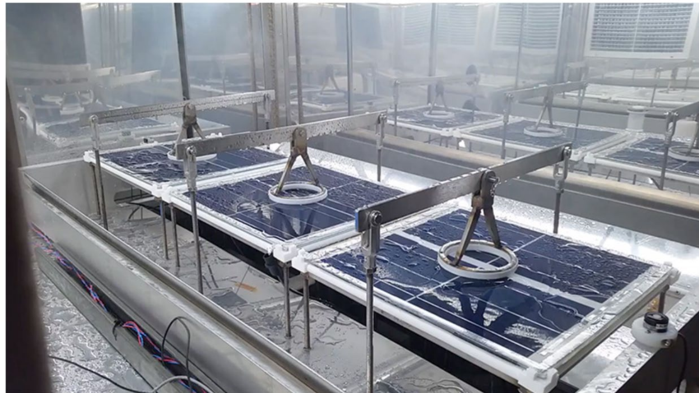
A screenshot from a video filmed by NREL researcher Peter Hacke shows the interior of one of the combined, accelerated testing chambers in Golden, Colorado. The "donut" rings periodically press down and flex the modules to provide mechanical stress, while the chamber subjects them to water, heat, cold, electrical loading, and ultraviolet light.
