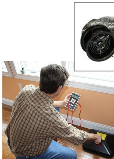
From top left: Duct Blaster ® Fan with Fan Speed Controller, Minneapolis Blower Door, and Pressure Pan.
